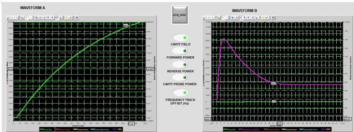
Fig.11: Lorentz force detuning illustration in Pulsed mode.
