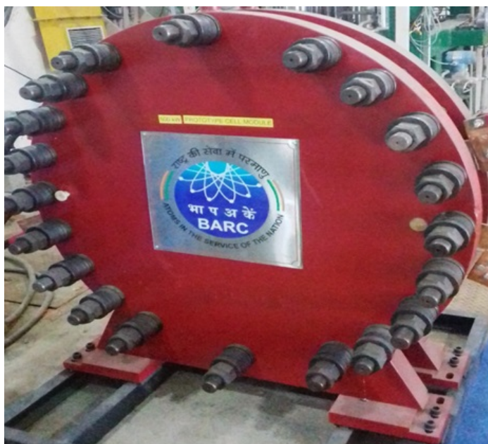
The Prototype 0.5MW Alkaline Water Electrolyser cell stack undergoing testing in BARC.
