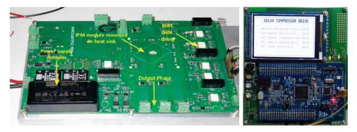
Fig.2: Power board with three leg IGBT Inverter module mounted on heat sink and Signal board with ARM based MCU unit, 3.2" LCD module and user interface.
