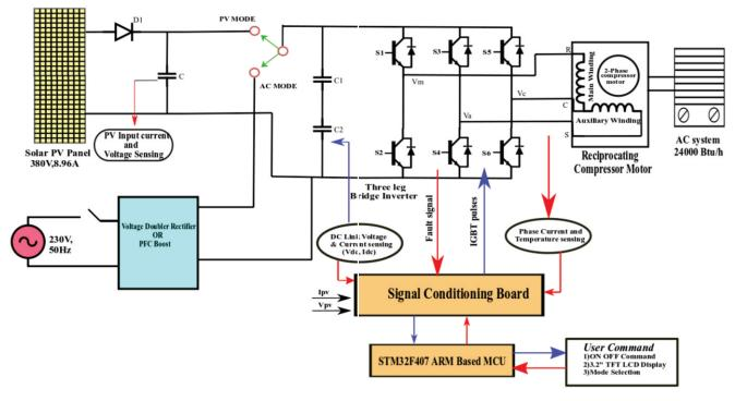
Fig.1: Block diagram of Air conditioning compressor drive powered by both solar power and 1-phase 230V, 50Hz AC supply.
