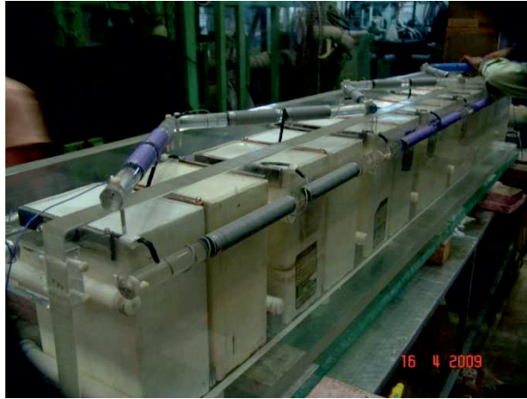
Figure 6.4. Photograph of 1kJ Marx generator.
