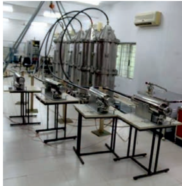
Figure 1.17. Marx generators with four channels of Flash X-ray sources designed for hydrodynamic studies.
