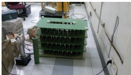
Figure 28.4: 84-Stage Marx Adder circuit with 50 k \Omega resistive load and 60 kV HV Probe.
