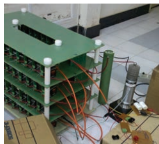
Figure 28.5: 84-Stage Marx Adder circuit from front showing 60 kV HV cable (orange colour).
