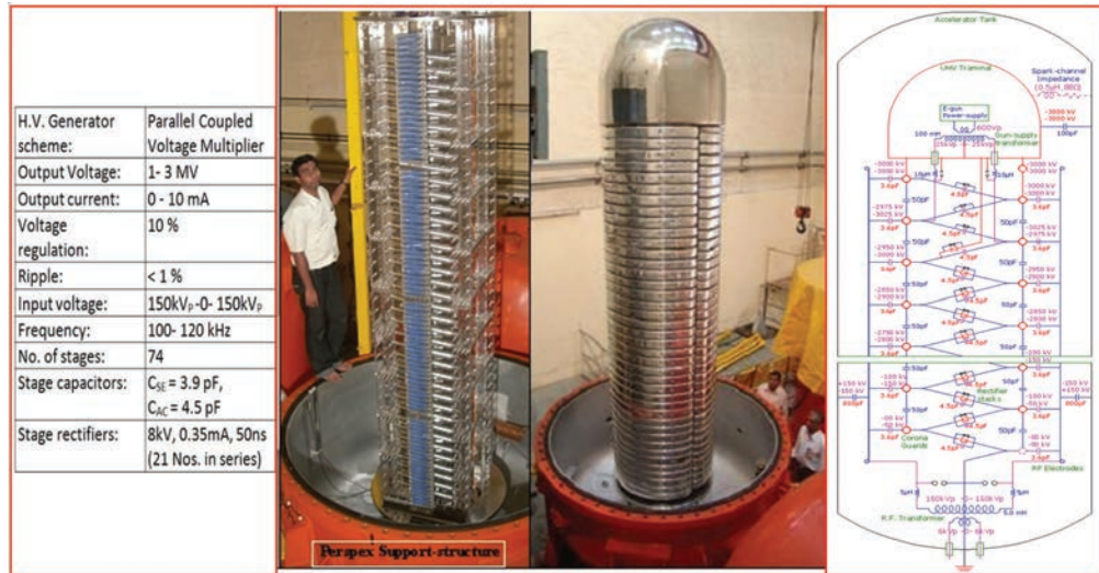
Figure 18.4: Specifications, 3MV multiplier photo & Electrical schematic of 3 MV generator.
