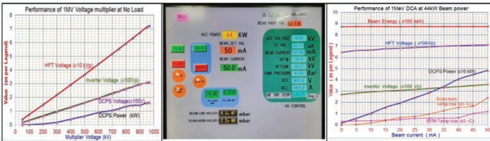
Figure 18.7: (Left) No Load, (center) HMI display, and (right) Load characteristics of 1 MV supply.
