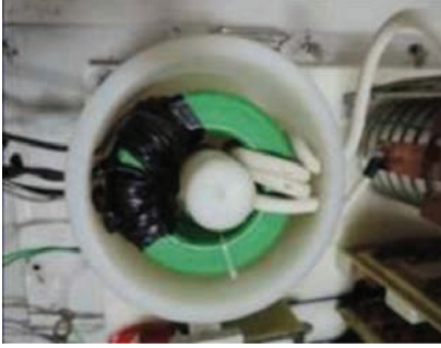
Figure 5.5: Transformer with toroid core.
